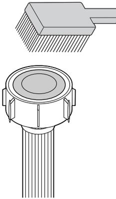
3. Refit the water supply hose to the tap and turn on the tap.
