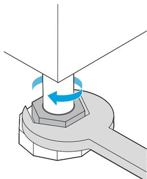
2. If any foot is not touching the floor: screw out the foot until it makes contact with the floor.
