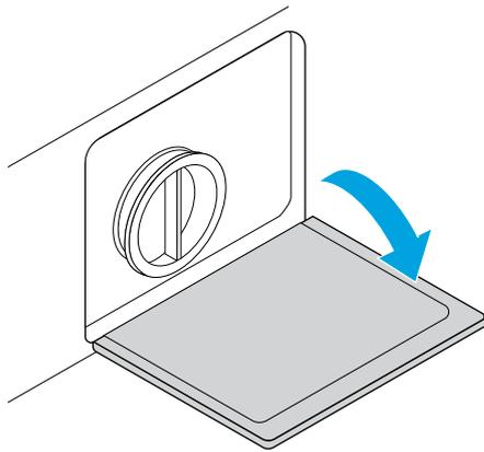
2. Rotate the filter anticlockwise and pull it out.
