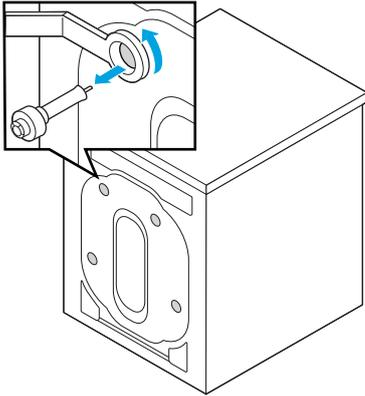
2. Plug the holes with the transport hole plugs.
