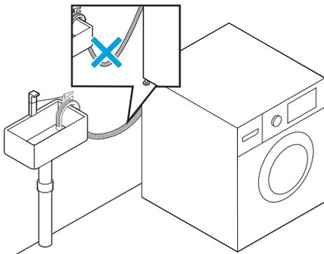
4. Secure the drain hose to the sink with a cord, clip or cable tie.
