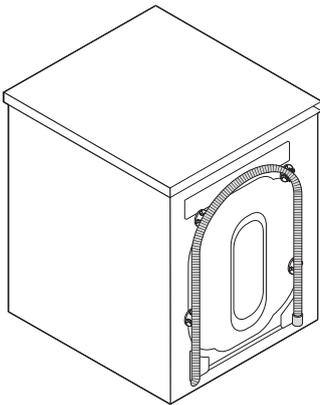
2. Insert the drain hose into the hose holder.
